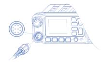
5. Plug the hand microphone (with direction sign at the top) into the corresponding interface of the radio, and rotate clockwise the cover lock on the plug. When the lock contacts the slot on the radio, press it slightly and continue to rotate until it is tightened.
